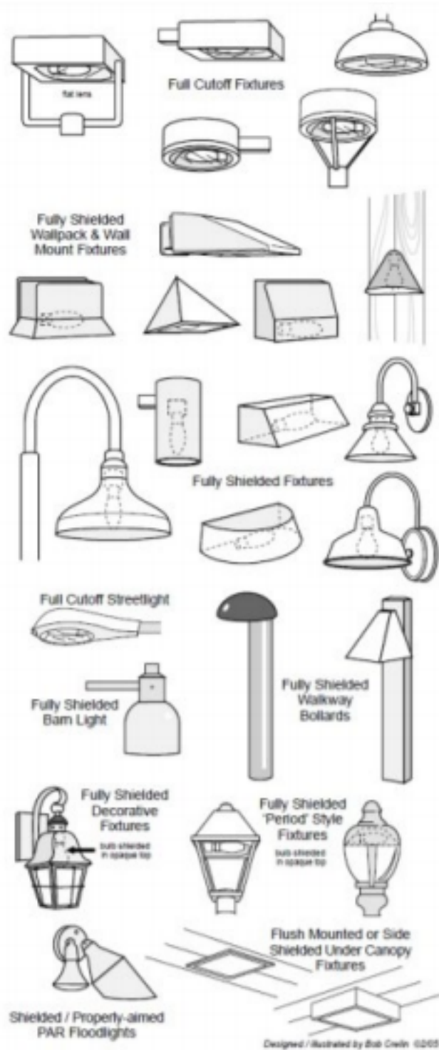
Figure 551-8: Examples of fully shielded and cutoff luminaries
